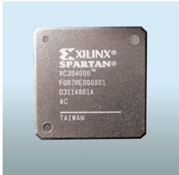
High-performance processor core based on programmable logic device
