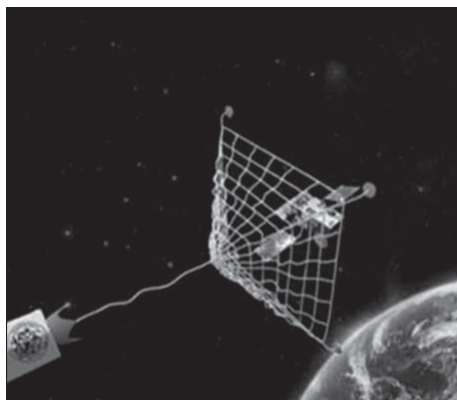
Fig. 1.3. An example of the special nets development with a cable connection for capturing SDO
