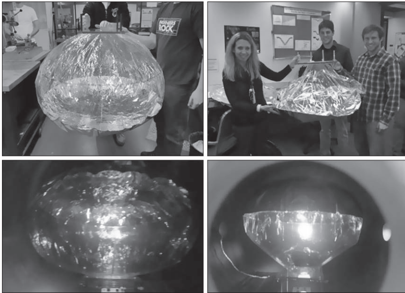
Fig. 1.7. Project of inflatable antenna for CommCube-1 spacecraft
