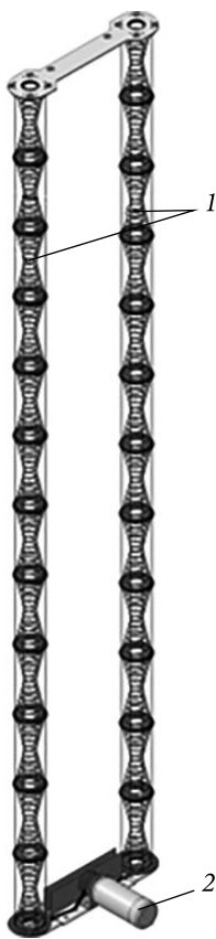
Fig. 4.11. Sail frame: 1 — spring mast; 2 — drive
