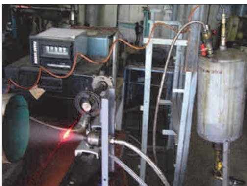
Fig. 5.45. Laboratory studies of the quality of nozzle spraying using a laser
