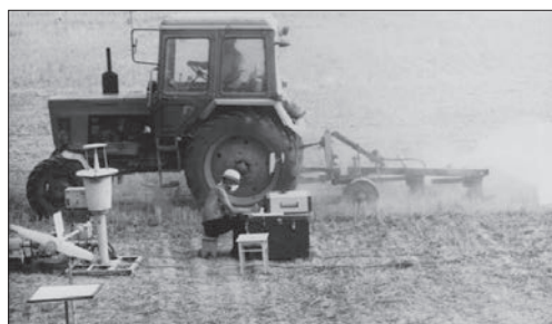
Fig. 2.4. Harrowing of the experimental ^{137}\text{Cs} contaminated strip with a T-150 tractor
