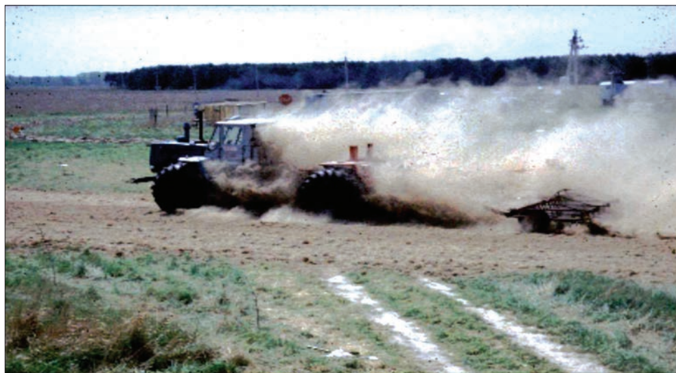
Fig. 2.4. Harrowing of the experimental ^{137}\text{Cs} contaminated strip with a T-150 tractor
