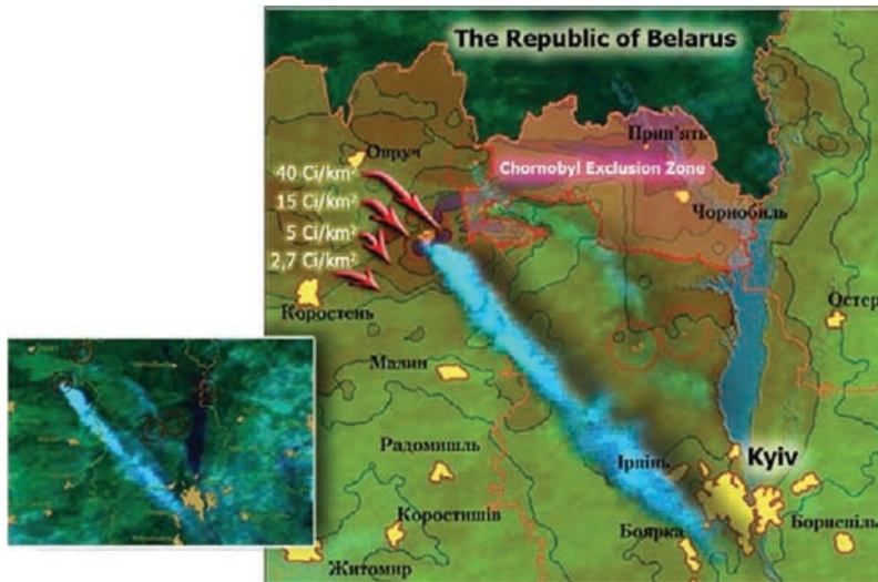
Fig. 14.2. Wildland fires in western Ukraine near the Chernobyl exclusion zone at territories with different ^{137}\text{Cs} contamination density ( 1 \text{ Ci km}^{-2} = 37 \text{ kBq m}^{-2} ) and smoke plume toward Kyiv, May 8, 2003 (from Goldammer et al. 2015)
