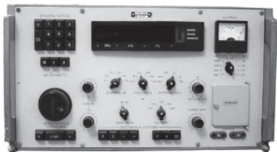
Fig. 3.3. Stationary superheterodyne short-wave radio receiver “Katran R-399A”
