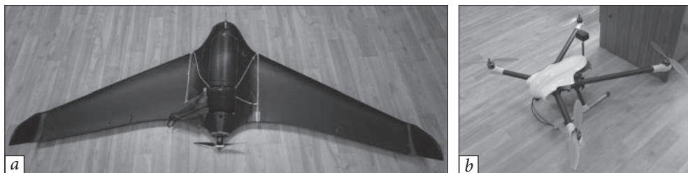
Fig. 2.8. The appearance of the UAV: a — aircraft type X-8, wingspan 2.12 m, estimated number of engine revolutions 8,000-11,000 rpm; b — quadcopter, estimated number of engine revolutions 6,000—10,500 rpm
