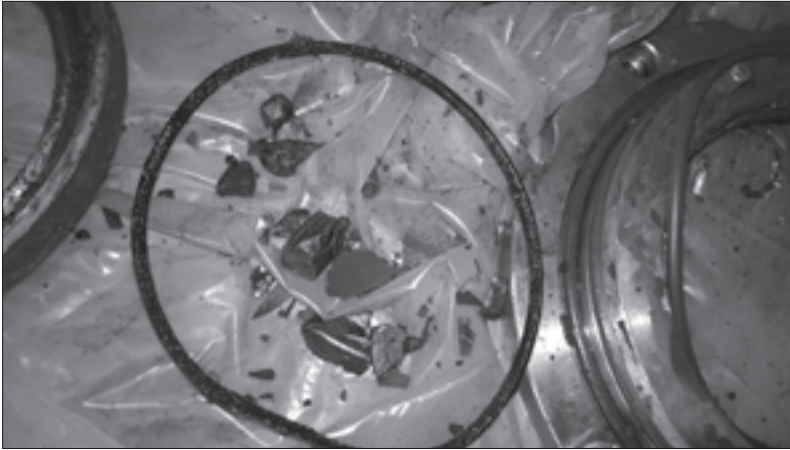
Fig. 7.14. Destruction of rubber rings
