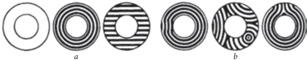
Fig. 5.4. Interference fringe patterns when measuring the flatness of ring surfaces using PI glass plates: a — normal plane; b — fine-tuning is needed
