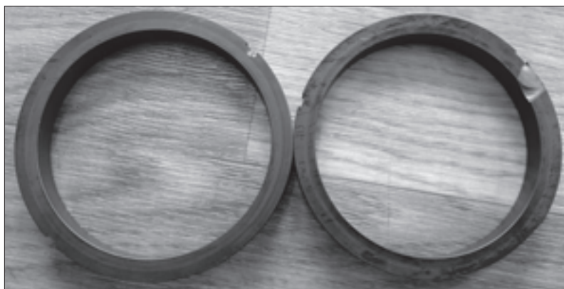
Fig. 7.9. Destruction of friction pair rings
