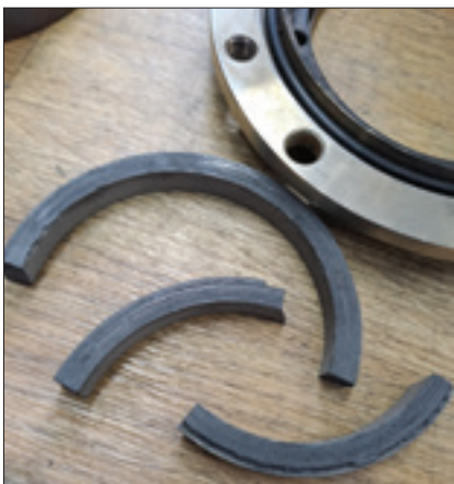
Fig. 7.3. Fragments of sealing rings with wear
