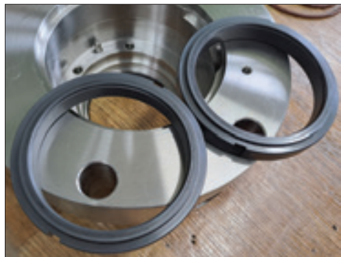
Fig. 7.4. Wear of the sealing strips of the end pair
