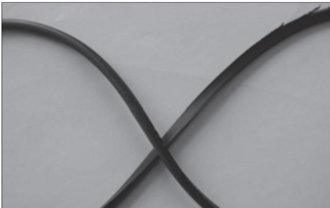
Fig. 7.16. Thermal destruction of rubber rings
