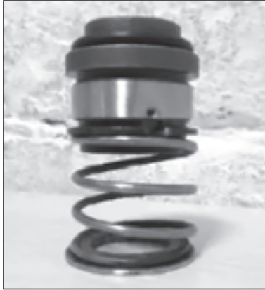
◀ Fig. 6.23. Typical single mechanical seal for the oil pumps
