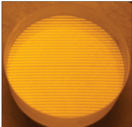
Fig. 5.2. Scheme for measuring the flatness of the surface of rings using a glass plate PI
