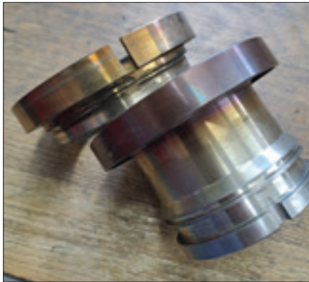
Fig. 7.5. Results of thermal effects on the rotor hub and cage
