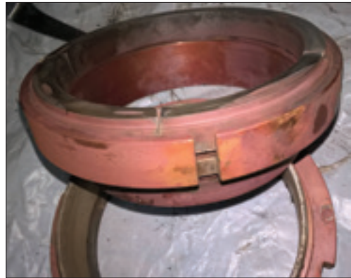
Fig. 7.6. Clip with a destroyed ring
