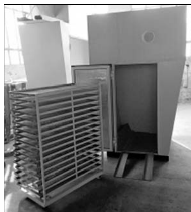
Fig. 1.14. Convective dryer with air recirculation
