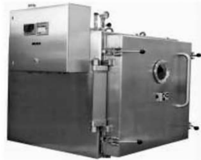
Fig. 1.16. Vacuum drying cabinet
