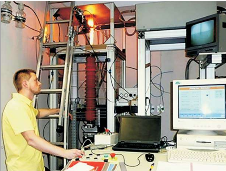
Fig. 2.15. General view of the growth setup during micro-PD fiber growth. The crystallization process is monitored using a CCD camera
