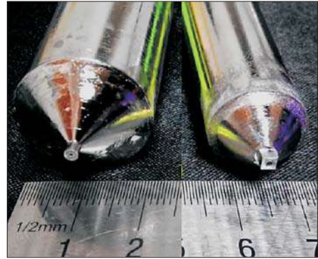
Fig. 2.20. Ir crucibles with a round capillary with a diameter of 2 mm (left) and a square capillary 2 \times 2 \text{ mm}^2 (right) [146]
