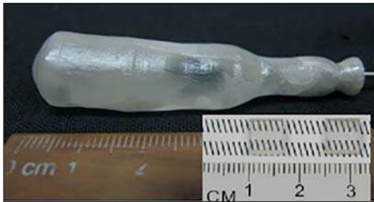
Fig. 2.10. Photo of grown GTNO crystal and fabricated samples for optical and scintillation measurements
