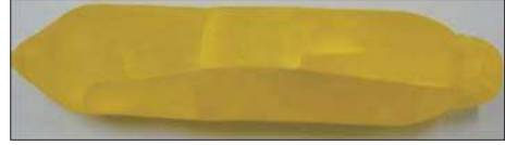
Fig. 2.6. Cracks in the GAGG:Ce crystal that formed just after the crystal was discharged from the growth furnace
