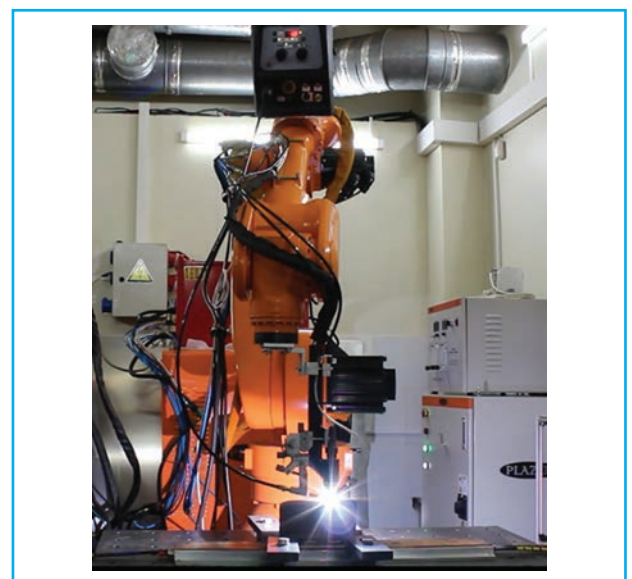
Robotic complex for additive plasma arc cladding of titanium alloy products in controlled atmosphere
