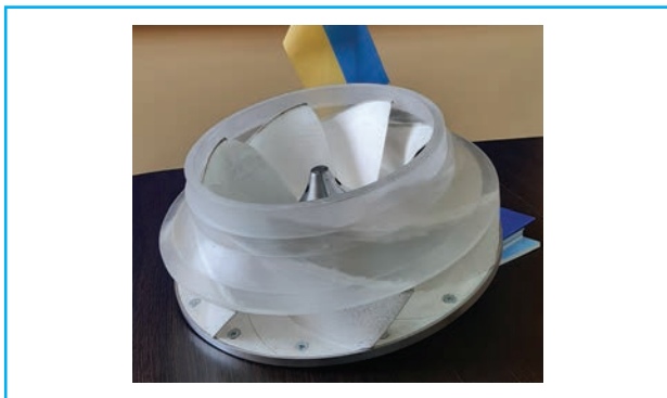
Model of PK5217M2 upgraded impeller of the Dniester PSPP turbine pump with improved energy and pulsation characteristics
